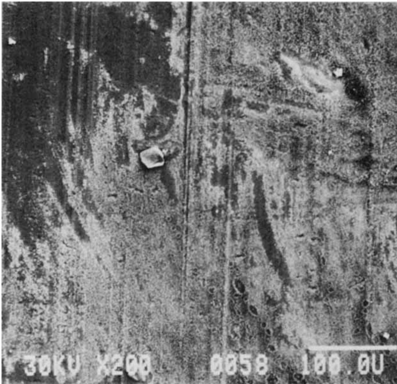
Fig. 8. SEM of HMDS coat prepared under the following conditions: frequency = 125 kHz, power = 100 W, monomer flow rate = 30 cm 3 /min, duration = 1 min.
